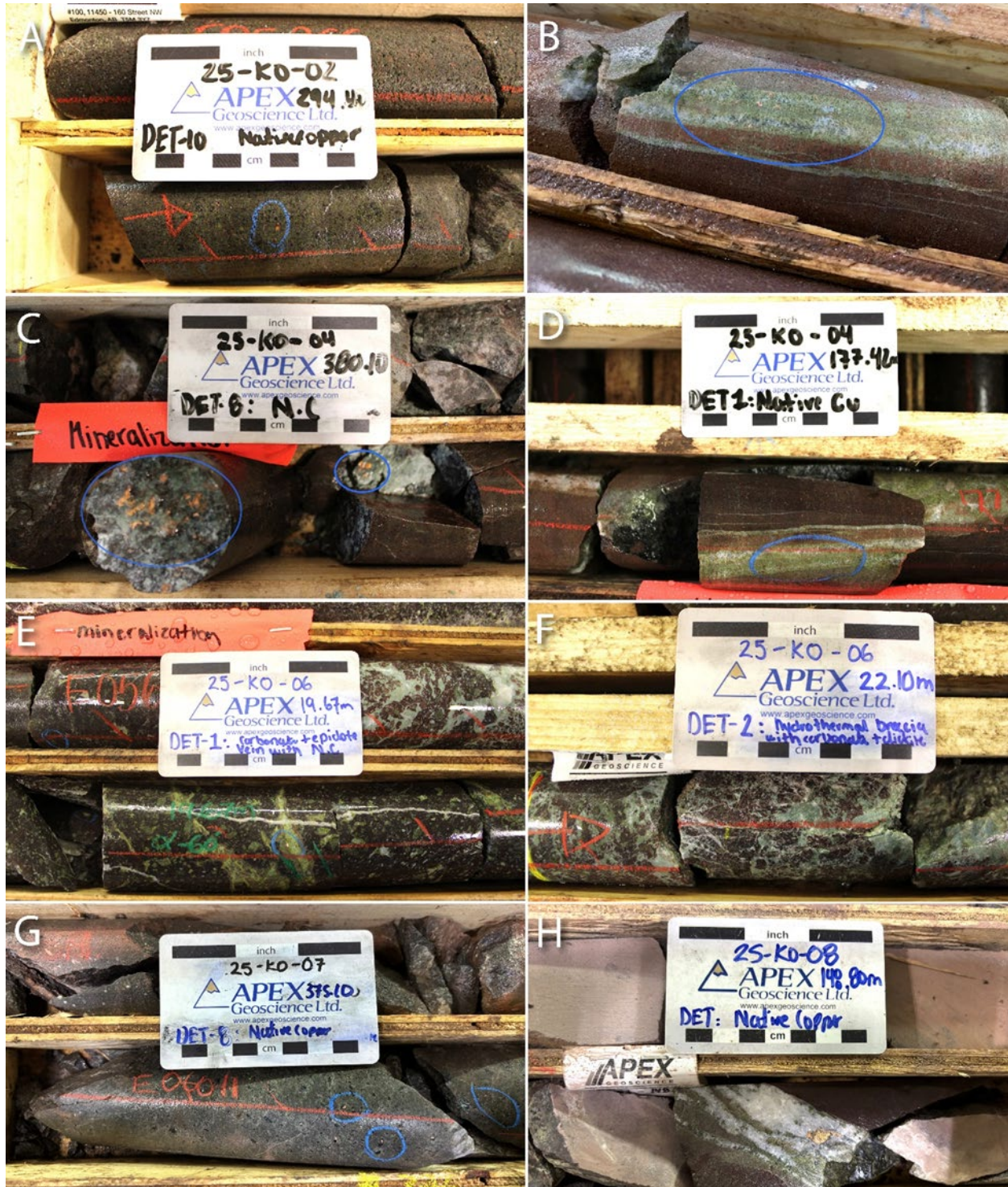
Figure 3. Select 2025 core photos. A. Native copper replacing mafic minerals in picrite. B. Native copper in epidote-carbonate veins hosted in hematized andesite. C. Native copper along chlorite filled fracture. D. Same as (B). E. Native copper in epidote-carbonate veins with hematite rims hosted in hydrothermal breccia in proximity to Bertha exploration pit. F. Hydrothermal breccia with carbonate cement \pm dickite (teal clay mineral) \pm epidote. G. Native copper replacing mafic minerals in picrite. H. Native copper in epidote-carbonate veins hosted in hematized andesite.
